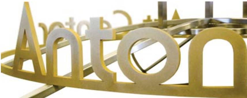
1/2" Waterjet cut bronze graphics mechanically mounted to a tig welded ring.
