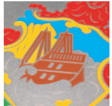
Waterjet cut, etched multi-coloured infilled st.stl. plate
