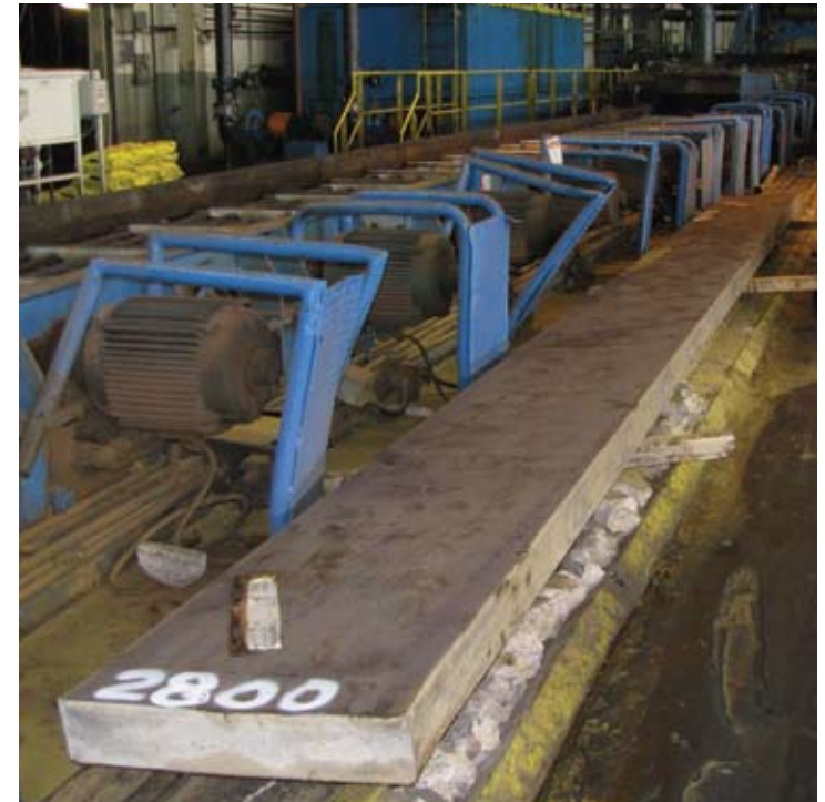
A Muntz metal (C28000) ingot, sometimes called a "cake", positioned alongside a furnace where it will be processed into roll form.
